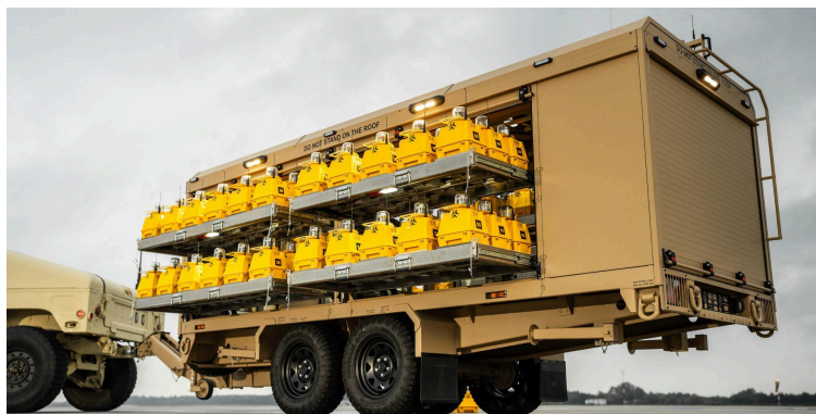
S4GA portable airfield lights in a trailer
