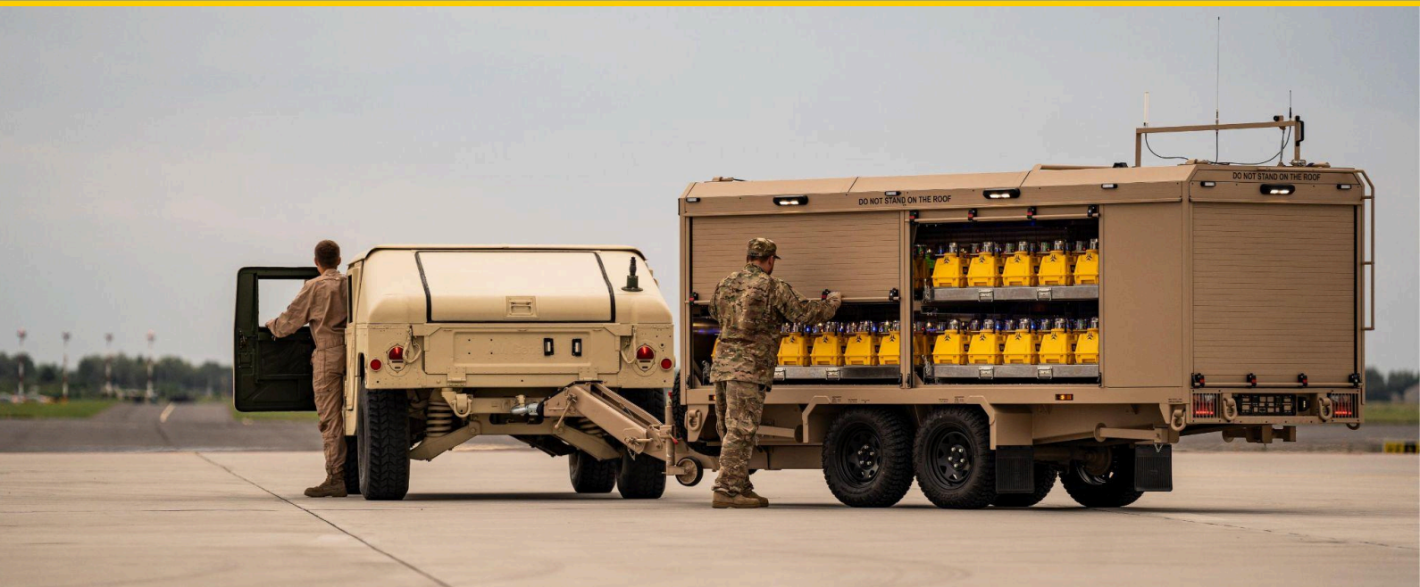
S4GA military airfield lighting trailer
