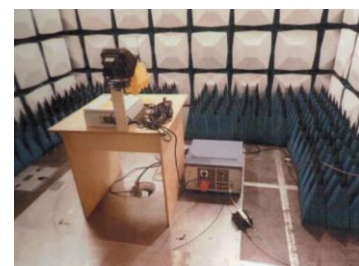
Figure 1.8. SP-401 Airfield Light during EMC testing in Military Institute of Armament Technology
