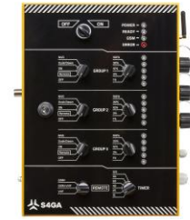
Figure 1.2. UR-201 Control & Monitoring Unit (hardware of S4GA ALCMS)
