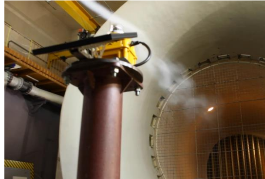
Figure 1.5. SP-401 Solar Airfield Light during testing of jet blast resistance in Warsaw Institute of Aviation
