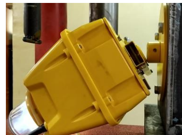
Figure 1.6. S4GA Frangible coupling during testing of frangibility in Institute of Research and Certification
