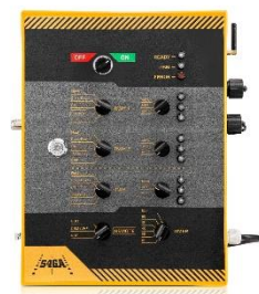
Figure 2.2. UR-201 Control & Monitoring Unit (hardware of S4GA ALCMS)
