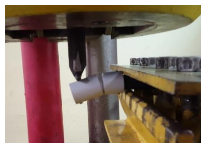
Figure 1.6. S4GA Frangible coupling during testing of frangibility in Institute of Research
