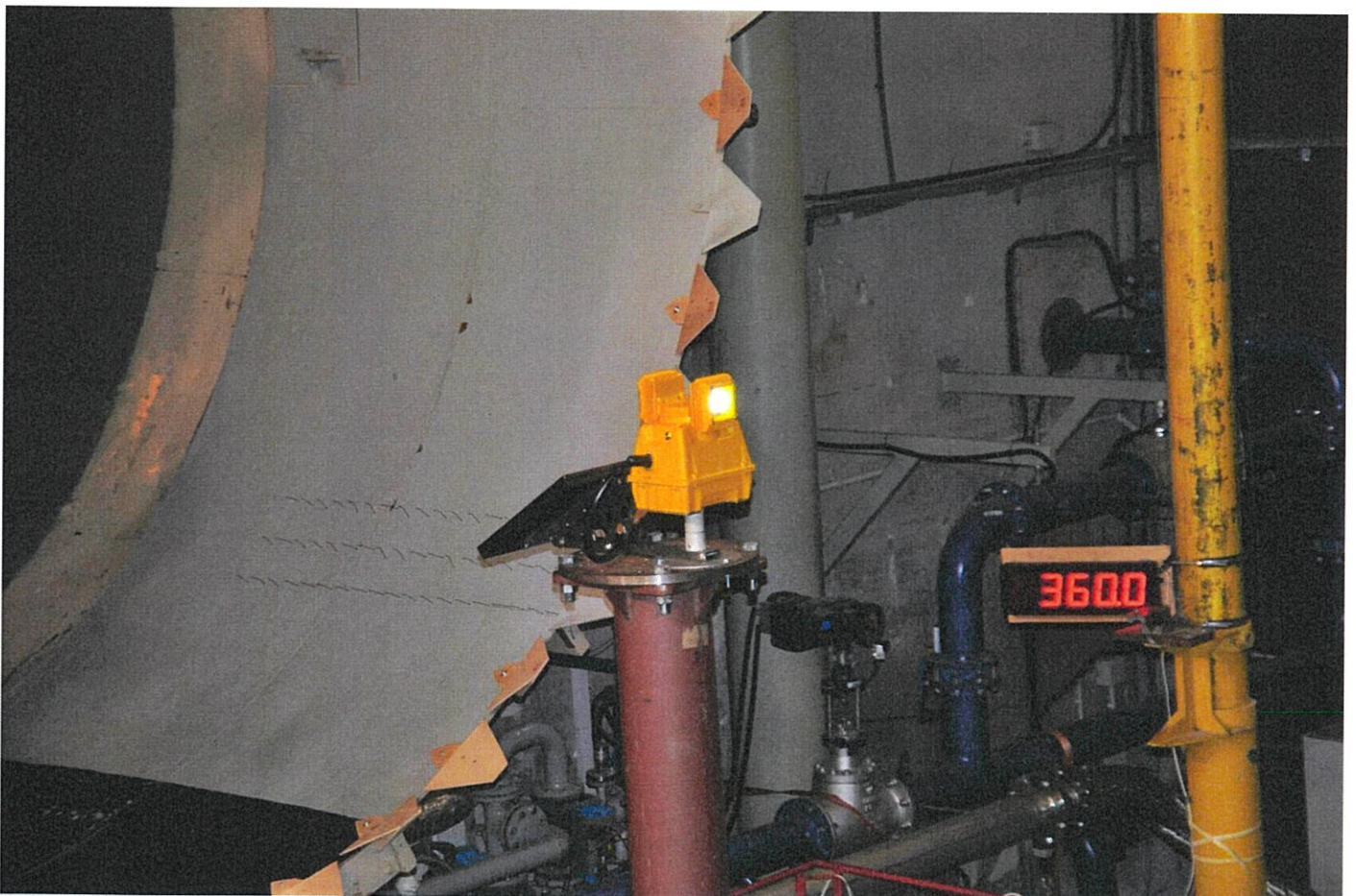
Figure 3 The SP-401 HIRL lamp with solar panel mounting on the test stand in the T-3 wind tunnel
