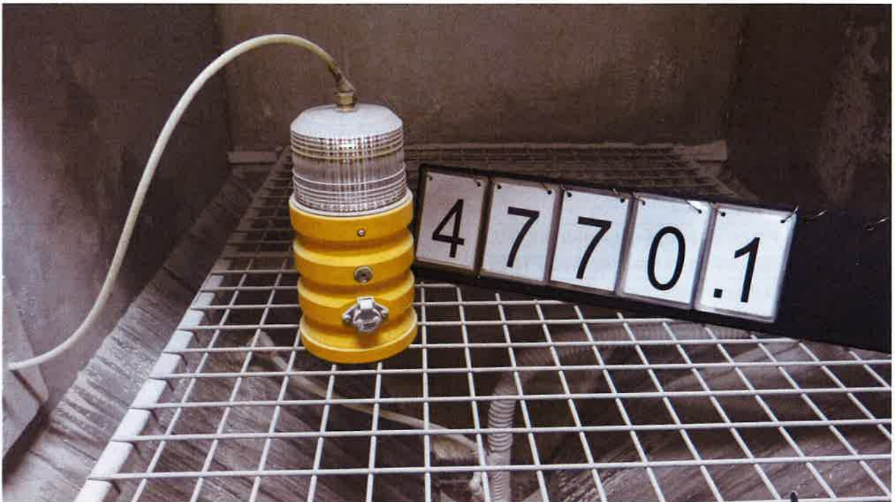
Fig. 1. Test sample 4770.1 in the dust chamber – after the test IP6X
