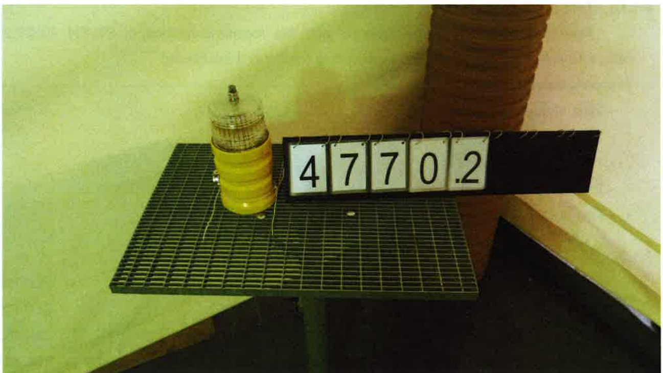
Fig. 2. Test sample 4770.2 at the test stand - after the test IPX5
