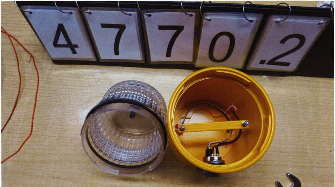
Fig. 4. Visual internal inspection after the test of IPX5. EUT – 4770.2/2017
