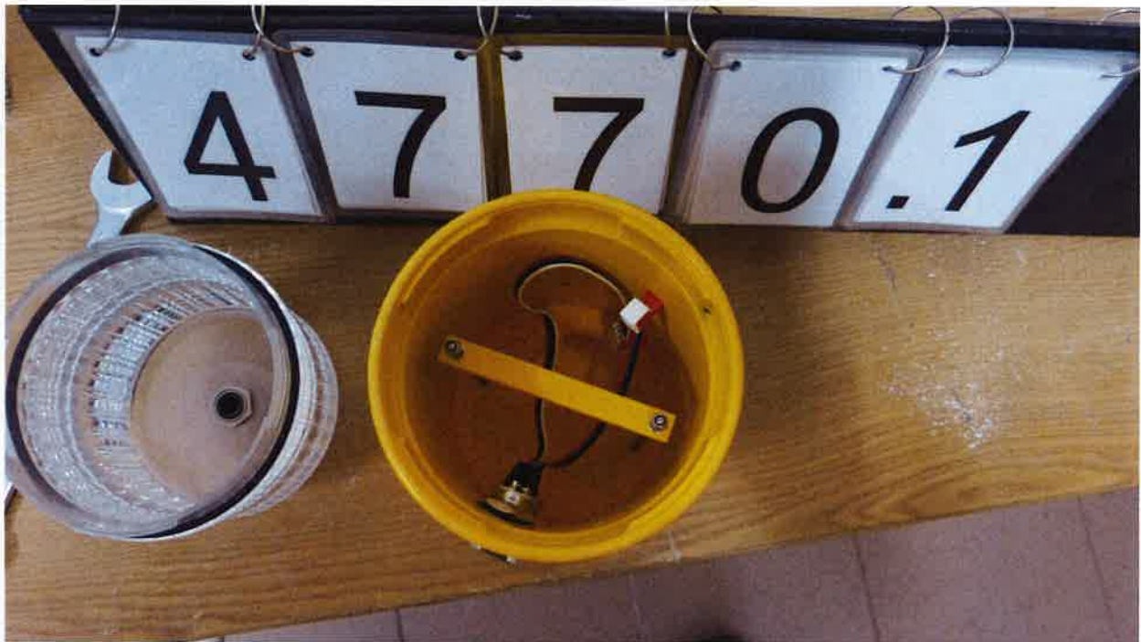
Fig. 3. Visual internal inspection after the test of IP6X. EUT – 4770.1/2017
